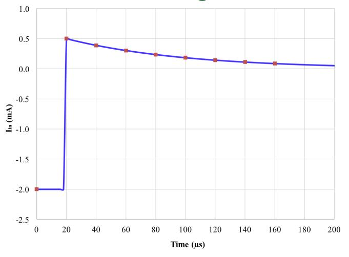
Current  $i_{in}[n]$  for Rser= -500 ohms, C= -0.1µF and T=20µs. Blue curve is continuous-time current, red dots are discrete-time current samples  $i_{in}[n]$
