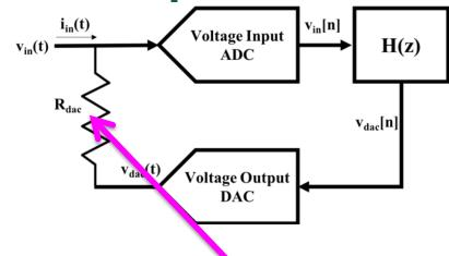
$$I_{in}(s) = \frac{V_{in}(s) - V_{dac}(s)}{R_{dac}}$$
