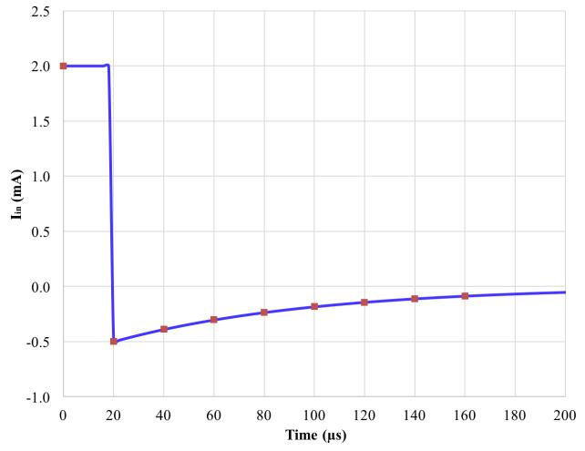
Current  $i_{in}[n]$  for Rser= 500 ohms, C= 0.1µF and T=20µs. Blue curve is continuous-time current, red dots are discrete-time current samples  $i_{in}[n]$
